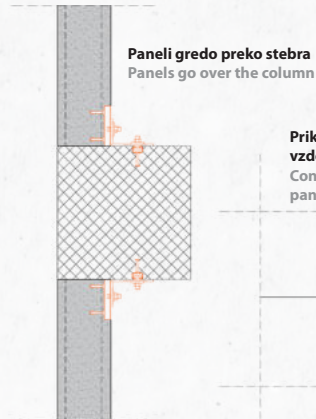
Prikaz povezave stebra in fasadnega panela v tlorisu (vidna povezava) Connection between the column and the facade panel in the base (visible connection)
